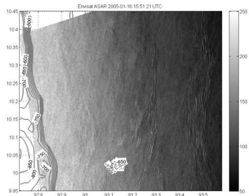
Figure 4. Envisat ASAR PRI dated 16.01.2005 acquired at 15:51 UTC over the Andaman Sea. Two wave trains with mode-2 structure are identified.
