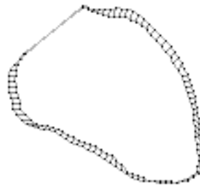
Figure 4.3 - Matching between two different contours with different number of points using the algorithm of dynamic programming (From Oliveira and Tavares, 2008).
