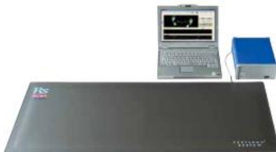
Figure 2.1 - An example of a RSscan Footscan fixed platform (From footscanusa.com).
