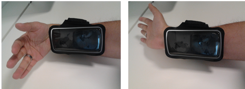
Figure 3.8: Wrist rotation to the left and to the right that can not be detected by the smartphone placed on the forearm.
