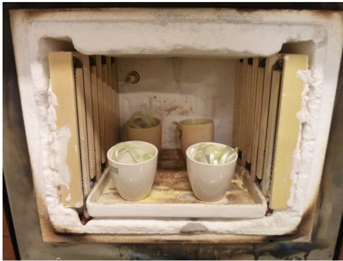
Figure 124 – Crucibles containing cured samples of impregnated fibre tows in the muffle oven before burn-off test start.
