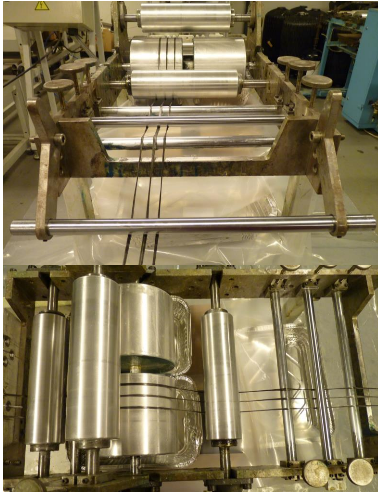
Figure 127 – Resin impregnation bath setup with double impregnation paths. Front (top) and top (bottom) views.
