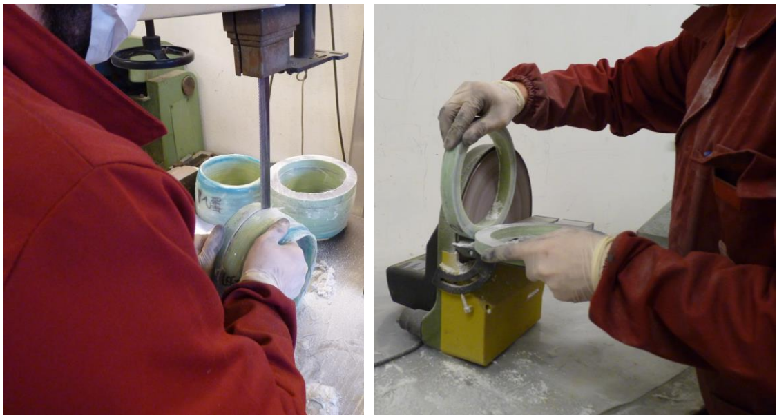
Figure 135 – Operations of transverse cutting of the wound specimens (left) and sanding of the cross-section surface (right).
