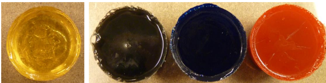
Figure 128 – Neat (left) and colorized resin samples. The black, blue and red samples correspond to the paste, liquid and powder colorizers, respectively.
