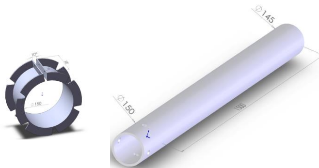
Figure 131 – Geometry of the mandrel and the de-moulding ring used in the winding trials.
