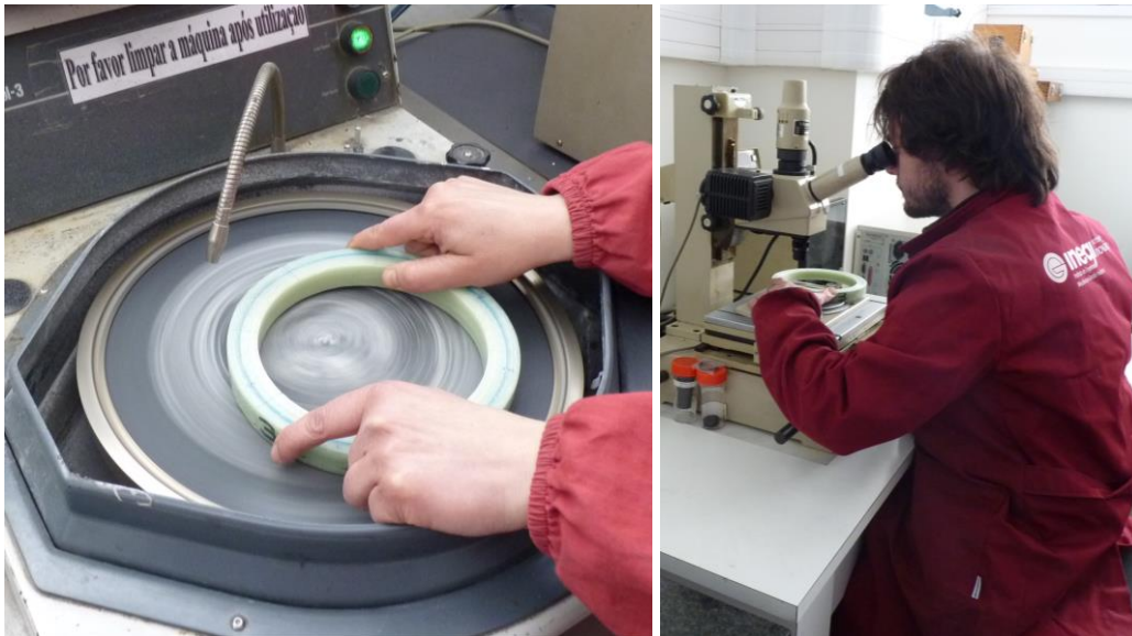
Figure 136 – Polishing of the cross-section measuring surface to enhance its readability (left) and microscopy measuring setup (right).
