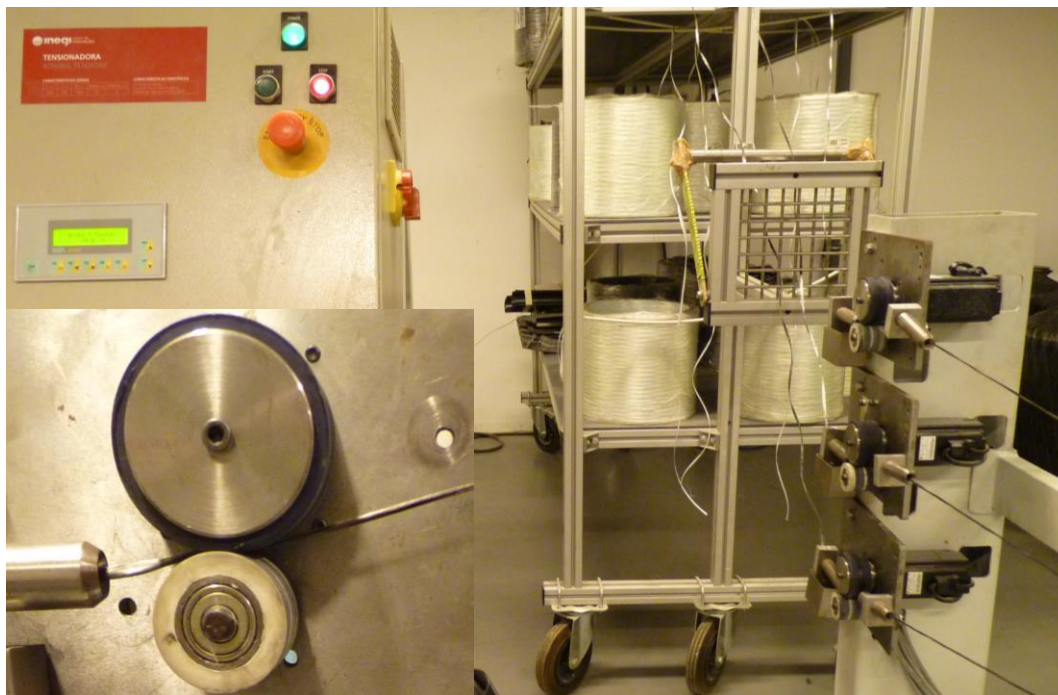
Figure 123 – Fibres tow pre-tensioning device based on a double wheel slip-less system (left bottom).
