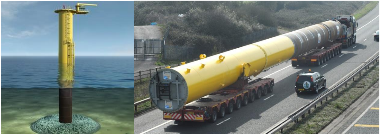
Fig. 2.9 – Monopile installed (a) and its transportation (b)
