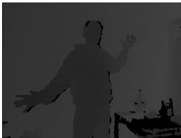
Figure 2.5 - Example of a raw depth image obtained using the Kinect (image from [28]).
