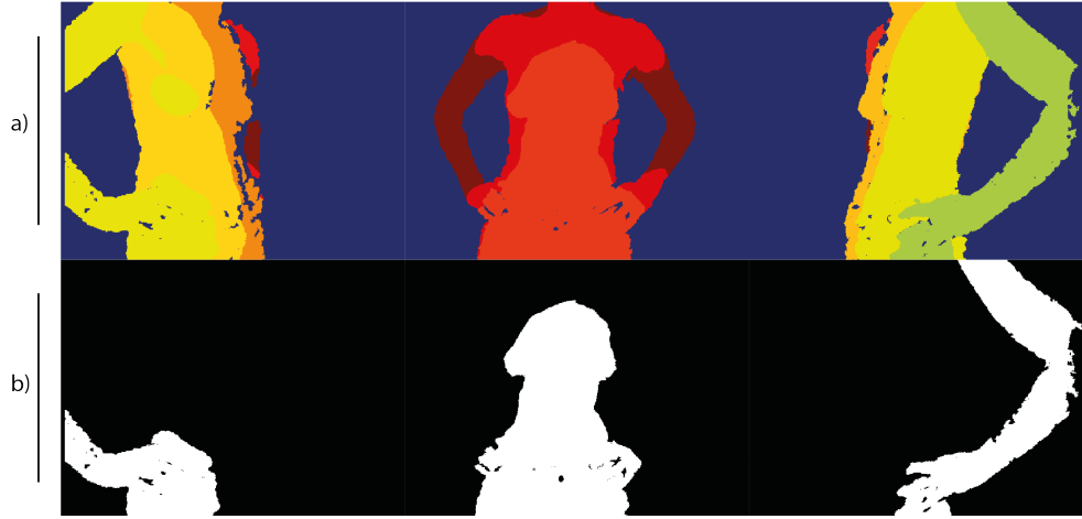
Figure 4.6: Closest Region Segmentation a) Results after applying the K-means Clustering method for segmentation, with different colors for labeling different regions; b) The closest region is segmented and isolated to measurement its area.
