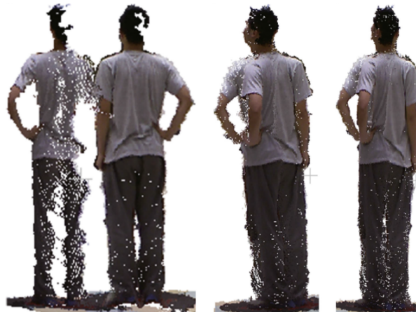
Figure 2.20: An example of a failure case of registration with two views resulting in a defective registration because of the variation position of the body (from [36]).
