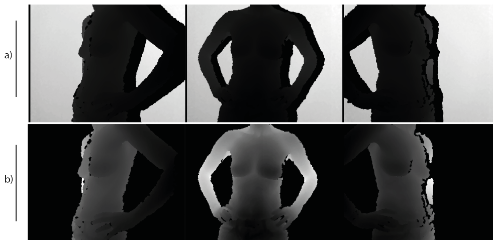
Figure 4.5: Background Removal. a) Examples of input normalized depth maps; b) normalized depth maps after applying otsu threshold and background removed.
