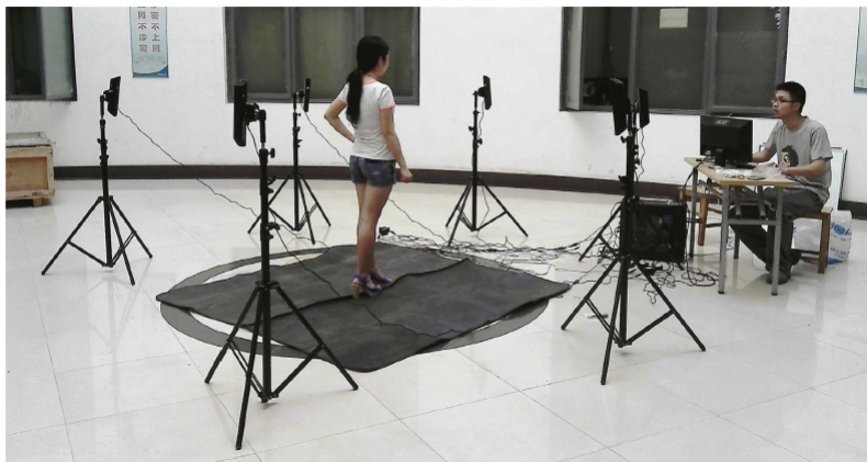
Figure 2.18: Environment of the experiment, where six depth cameras were placed around the user(from [36]).
