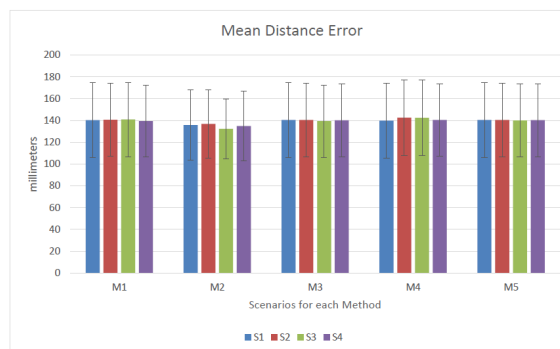
Figure 5.3: The average mean euclidean distances error (in millimeters) for each method and scenario, using the direction from the Microsoft Kinect model to the 3dMD model.
