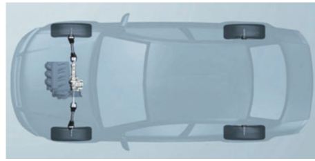
(a) Front-wheel-drive configuration
