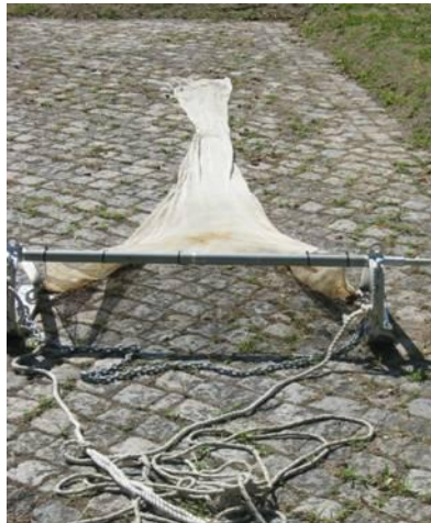
Figure 3: Beam-trawl used to collect the shrimps for the experiments
