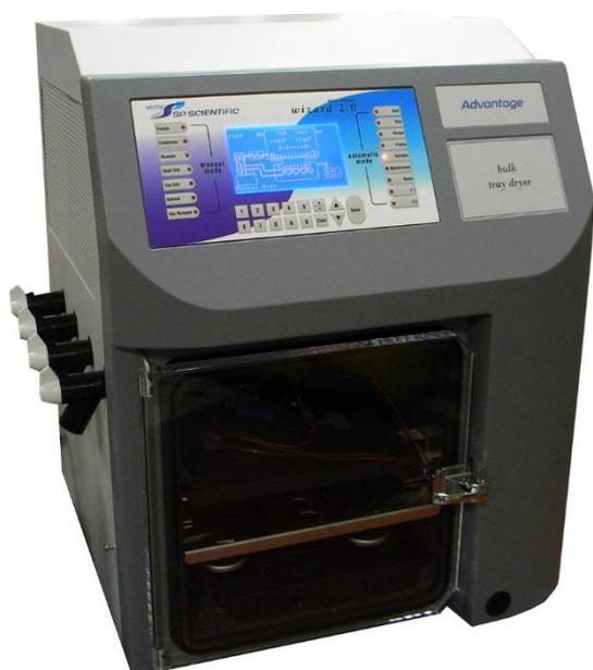
Figura 13: Aparelho AdVantage 2.0 Bench Top FreezeDryer, Virtis SP SCIENTIFIC [172].
