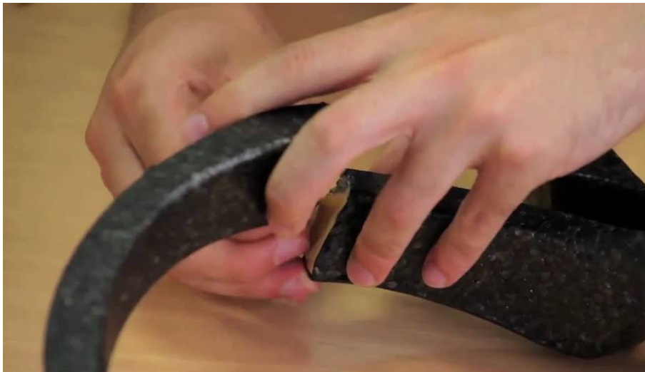
Figure 5.8: Repairing the external hull of the AR. Drone with a double sided adhesive tape
