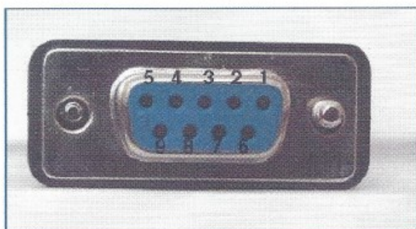
Pin layout for DB9 type connector on QM14BTF 14-Pin Butterfly mount
