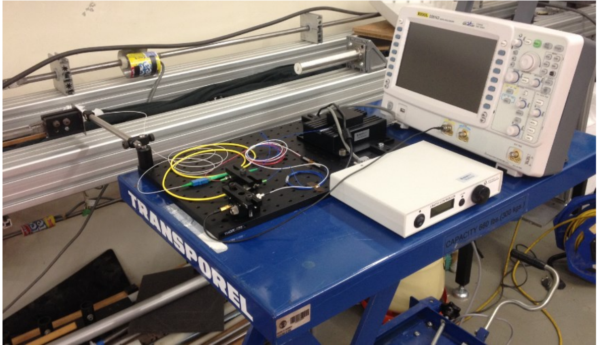
Figure 3.20 – Final assembly of PDV in the Hopkinson bar
