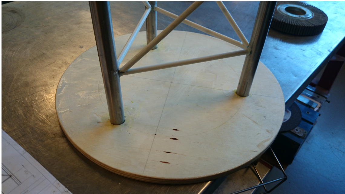
Figure 3.7: Base plates added to facilitate installation in wind tunnel.
