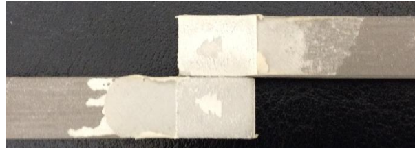
Figure 53. Failure mode after quasi-static testing of a SLJ with XNR 6852E-2 at low temperature (5 mm adherends; moist).
