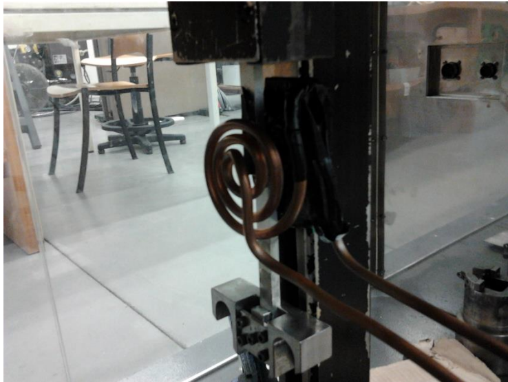
Figure 48. Single lap joint mounted and waiting to be heated up before a high temperature impact test.
