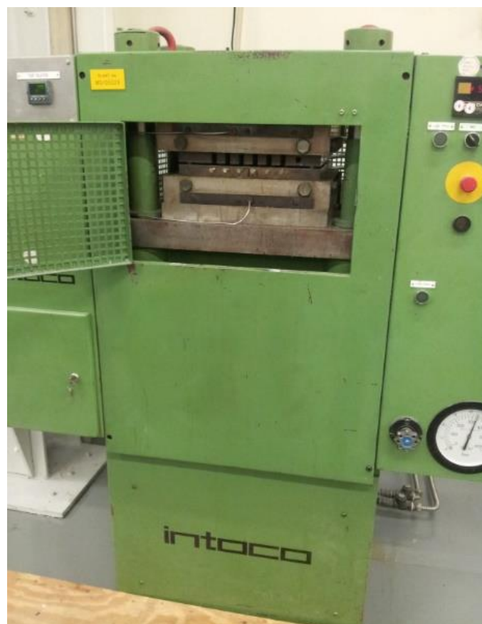
Figure 43. Hidraulic hot plates press with a mould inside.
