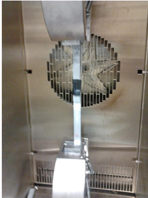
Figure 45. Single lap joint mounted for a quasi-static tensile test.
