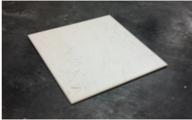
Figure 29. Bulk specimen for the XNR 6852E-2 water absorption test.
