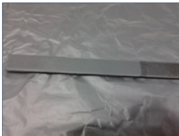
Figure 40. 2mm adherend after surface preparation (The left, lighter section has been anodized).
