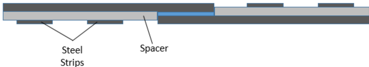
Figure 41. Positioning of spacers and strips relative to the joints in the mould.
