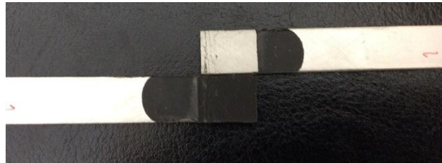
Figure 69. Adhesive failure under impact of a SLJ with SikaPower 4720 at low temperature (2 mm adherends; dry).
