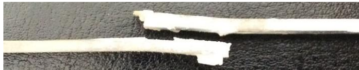
Figure 52. Adherend yielding after quasi-static testing of a SLJ using SikaPower 4720 with 2 mm adherends (-20 °C; moist)
