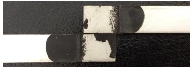
Figure 57. Adhesive failure after quasi-static testing of a SLJ with SikaPower 4720 at low temperature (2 mm adherends; dry).
