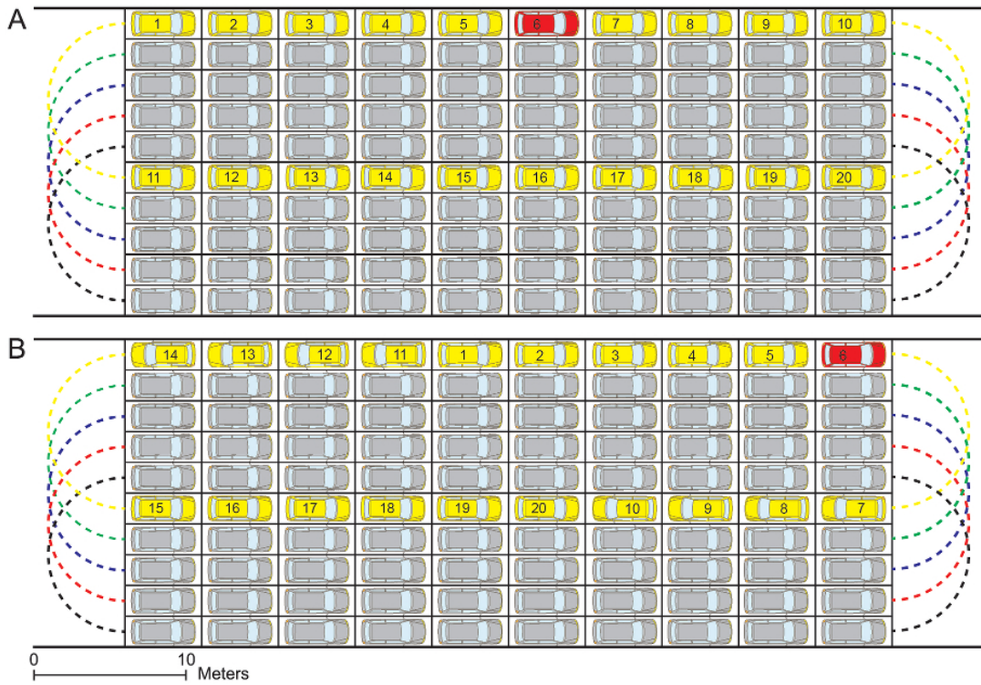
Figure 9.4: Completely full parking lot. In this architecture, vehicles use the buffer areas to implement carrousel between lines 1-6, 2-7, 3-8, 4-9 and 5-10. Rotation can be clockwise or counter-clockwise.
