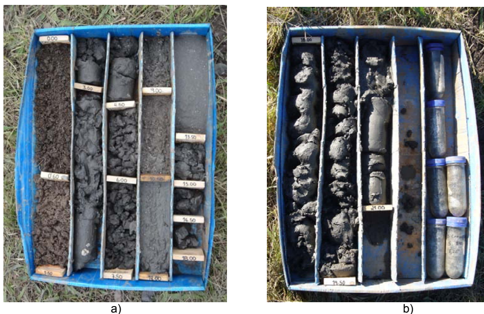
Figura 7.2 – Amostragem contínua perturbada: a) 0,0 m – 18,0 m; b) 18,0 m – 21,0 m.
