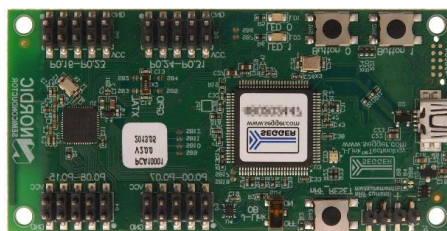
Figure 4.3: Nordic's PCA10001 development board [79]
