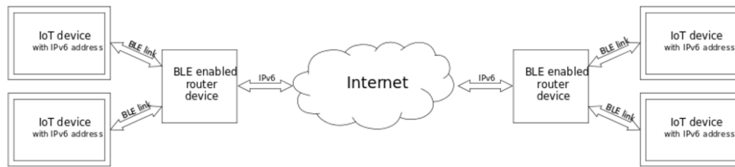
Figure 4.7: An example of an IoT network communicating by using BLE links with 6LoWPAN support [82]
