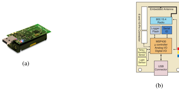
Figure 3.12: In Fig. 3.12a the TelosB module is shown, and its respective block diagram in Fig. 3.12b.
