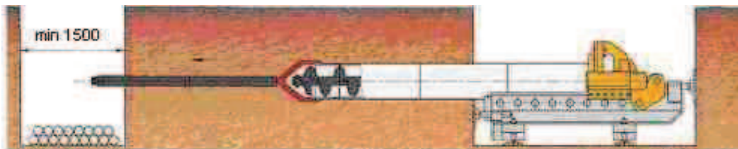
Fig. 2.11 – Thrust Auger Boring (Hidrossolo 2006)
