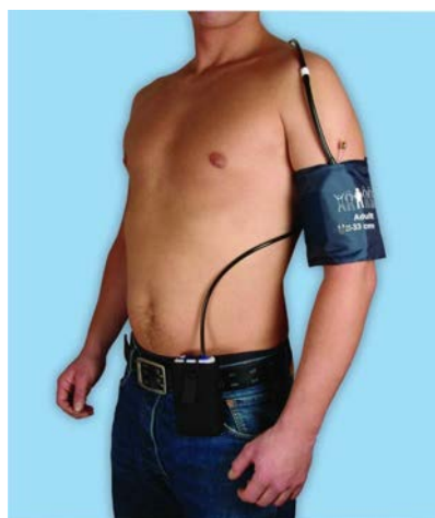
Figure 2.8: Arterial blood pressure monitor example (adapted from Farum ® S.A. SH-P ABPM device model).
