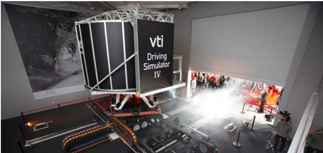
Figure 7: VTI driving simulator (hydraulic systems simulate vehicle motion) [34].
