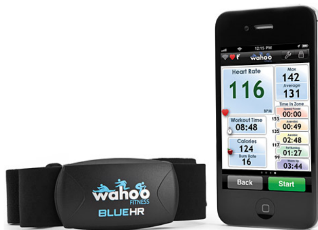
Figure 2.6: Wahoo Blue HR sends physiological data to the smartphone wirelessly 4
