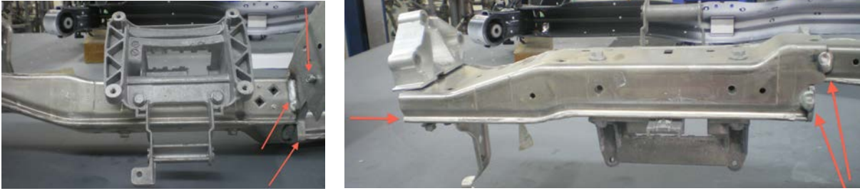
Figure 3-35- Several photographs of an aluminium CCB from a VolksWagen Passat of 2007 (SODECIA 2012)
