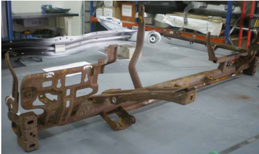
Figure 3-32 – A steel CCB from a BMW Serie 3 illustrating the complexity of some steel solutions with their multitude of support brackets welded to the main structural element (SODECIA 2012)
