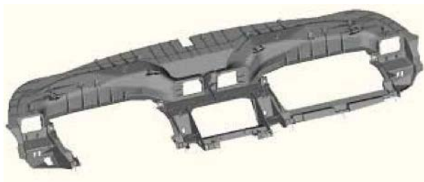
Figure 3-46 – the upper IP frame of the hybrid cockpit structure (Jahn et al. 2004)
