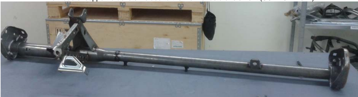
Figure 3-33 – A steel CCB from a Citroen C1 illustrating a very simple example made from two different tubular sections that are welded together (SODECIA 2012)
