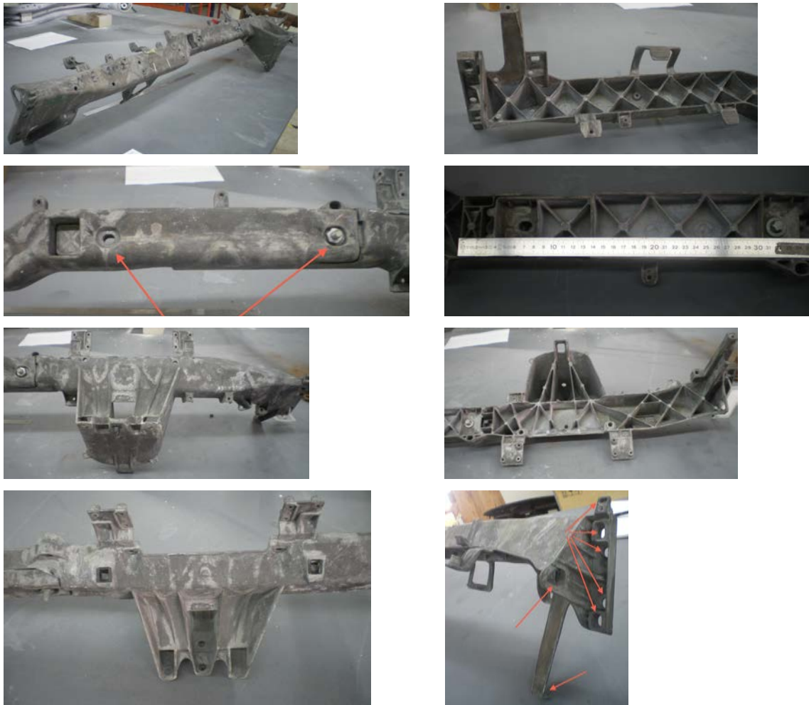
Figure 3-34- Several photographs of different perspectives of a magnesium CCB from a Mercedes Class E of 2007 (SODECIA 2012)
