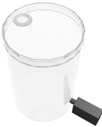
Figure 3.3 – The decellularization agent container and valve, after rendering
