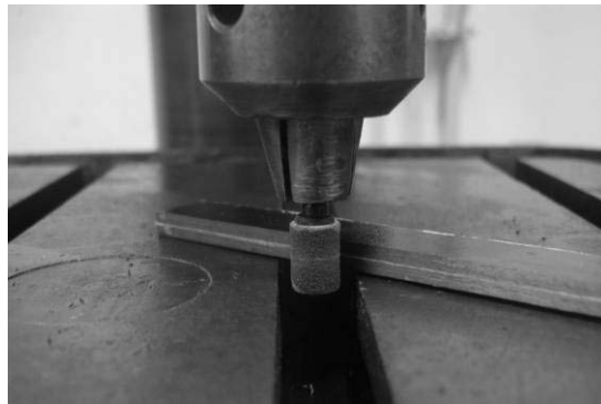
Fig. 74 – Finishing of a specimen in a drilling machine with a spiral band.
