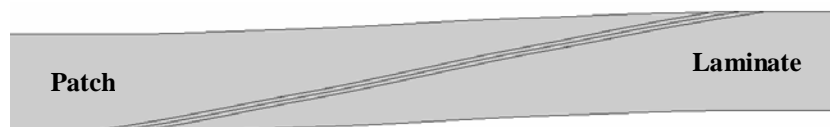
Fig. 270 – Deformed configuration of the scarf repair under a tensile load (2D repair).
