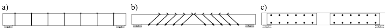
Fig. 60 – Repair methods tested in the wood beams fractured by horizontal shear (Akbiyik 2005, Akbiyik et al. 2007).
