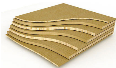
Figura 2. 11 - Folheado ("veneer plywood") [13]
