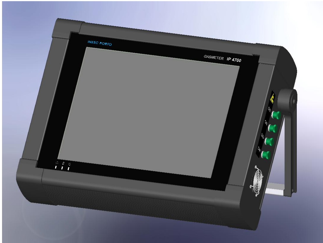
Figure 98 – 3D computer model of the portable monitoring unit that is being implemented
