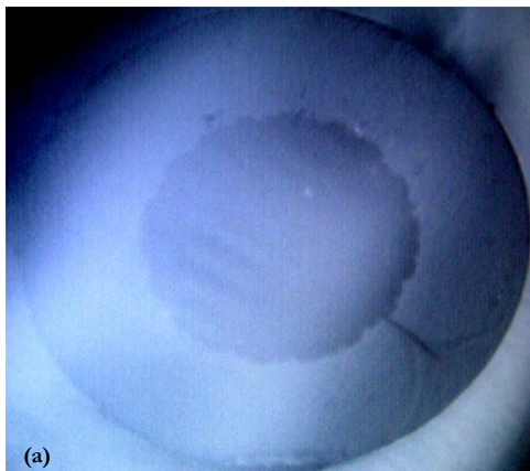
Figure 91 – Photos taken with a microscope of the HC-PCF position inside of the ferrule: (a) HC-PCF with an outer diameter of 125\ \mu\text{m} ; (b) HC-PCF with an outer diameter of 115\ \mu\text{m} .
