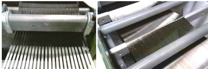
Fig. 2.8. Thin plies obtained with the tow spreading technology at Chomarat.
