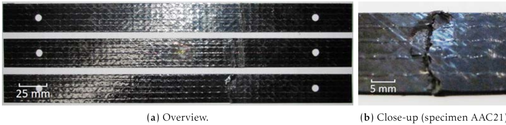
Fig. 4.10. Thin-ply [(0/-45)/(45/0)/(90/45)/(-45/90)] S specimens after compressive plain strength testing.
