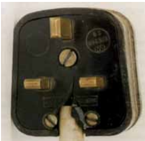
Cracked casing and damaged cable sheath
