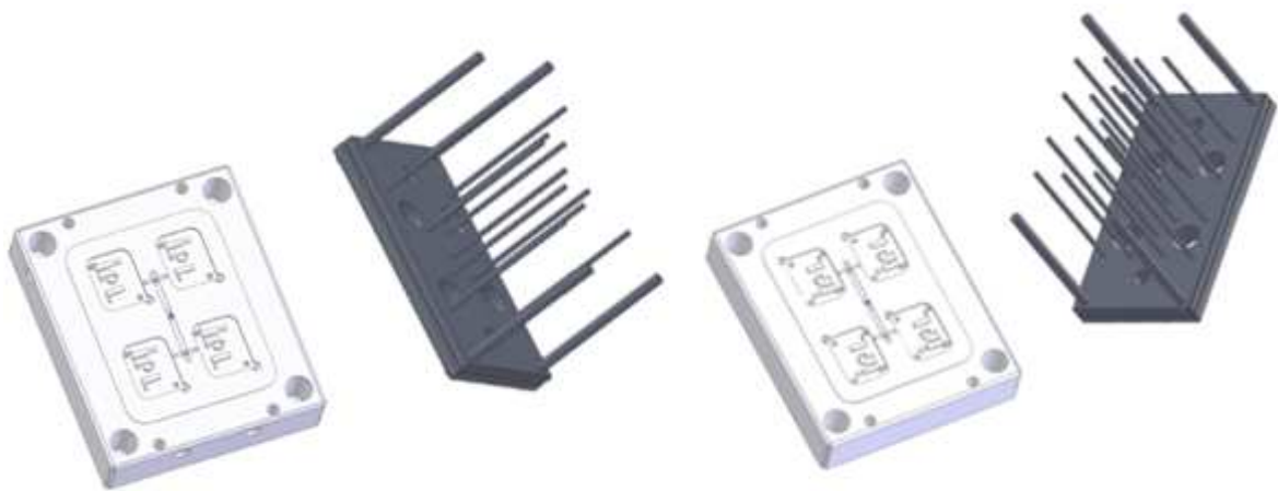
Figure 4.47: The two possible alternatives for n Ejectors : two pins per part (left) or four pins per part (right).
