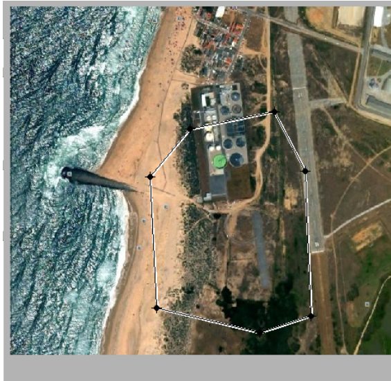
Figure A.7: Set the area to be surveyed by clicking and dragging
