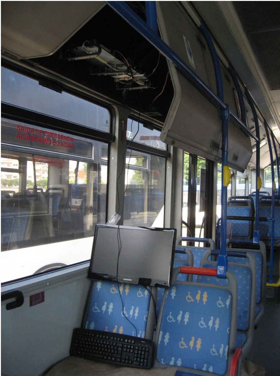
Figure 5.3: SITMe equipment mounted in a bus
