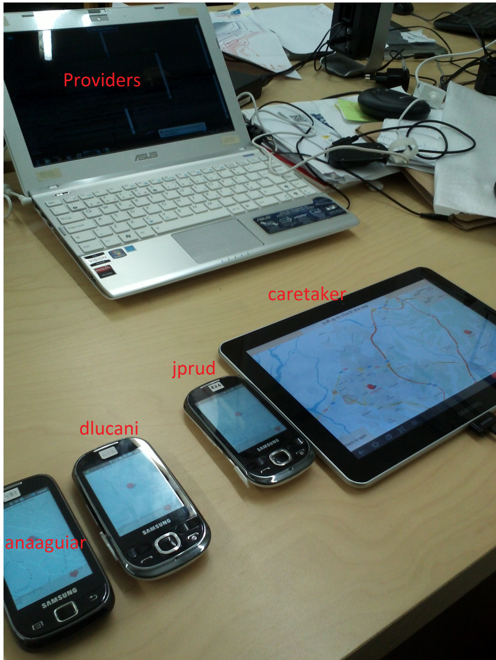
Figure 6.1: Test of the system developed, using two mobile phones as context sources, and another mobile phone and a tablet as context consumers.
