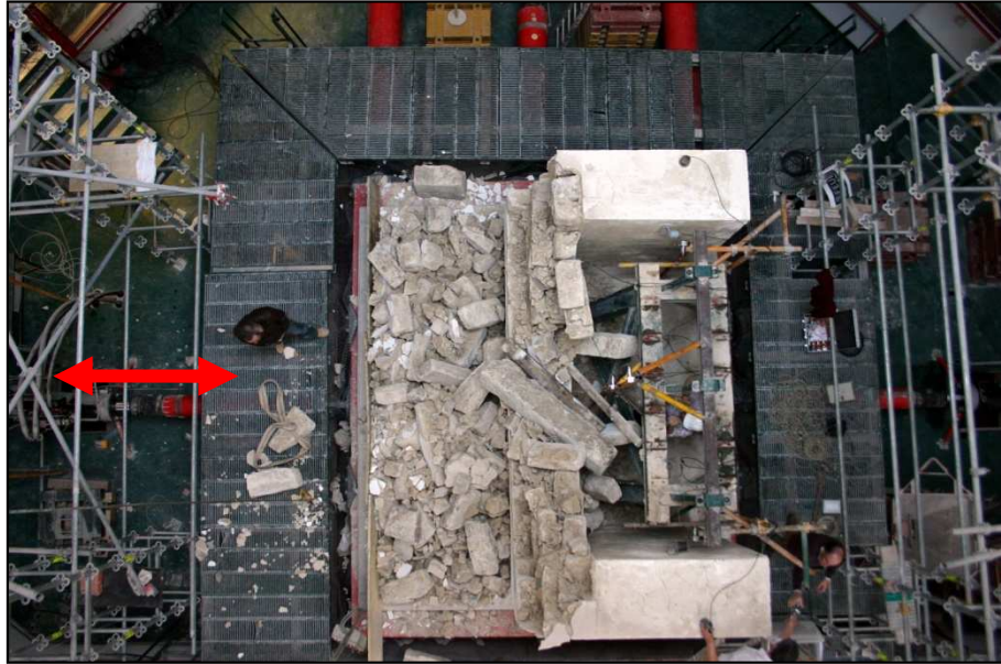
Figure 4.1. Top view of the LNEC triaxial shaking table with a specimen after collapse (H1 specimen), with representation of the transversal direction
