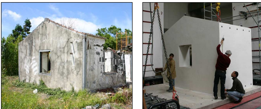
Figure 4.3. Masonry house façade reproduced on the shaking table tests: a) real existing building in Azores; b) specimen at LNEC shaking table
