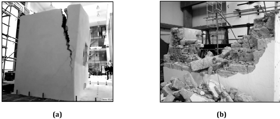
Figure 6.4. Collapse mechanism formed: a) global overturning; b) collapse picture at the end of the shaking table test L5-80% with leafs' step failure
