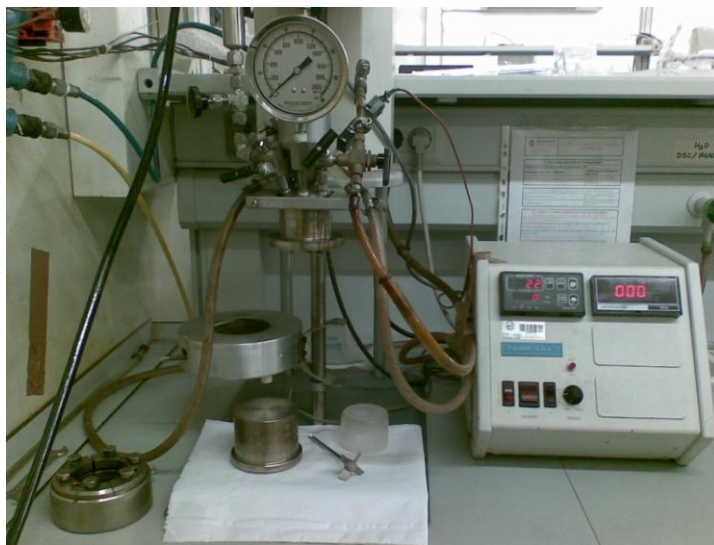
Figure 2.1 - Autoclave and temperature controller used in the functionalization of the SWCNT.
