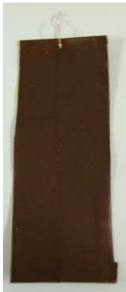
Figure 3.1: PVC band wrapped with tape A.
