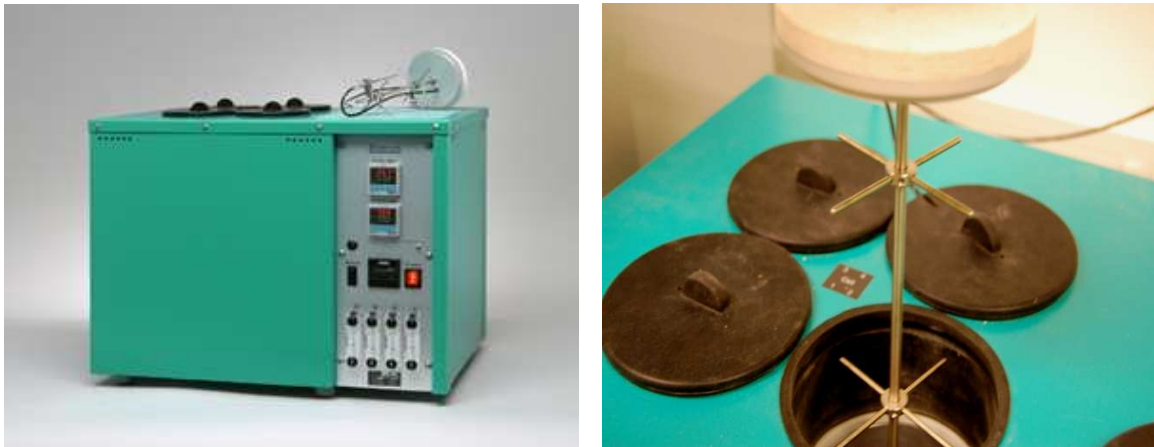
Figure 2.1: To the left: Cell oven EB01 from Elastocon. To the right: 4 oven cells.
