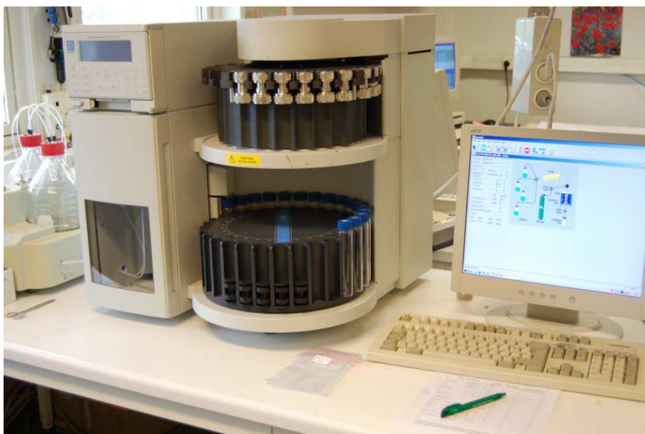
Figure 3.2: Dionex ASE 200 Accelerated solvent Extractor .
