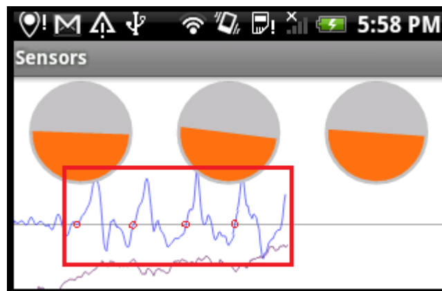
Figure 4.7: Acceleration measurements over four sequential steps, red circles represent the instants where footfall recognition is triggered
