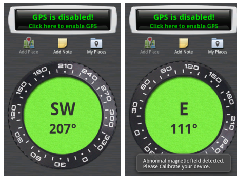
Figure 4.10: Magnetic interference in compass sensor
