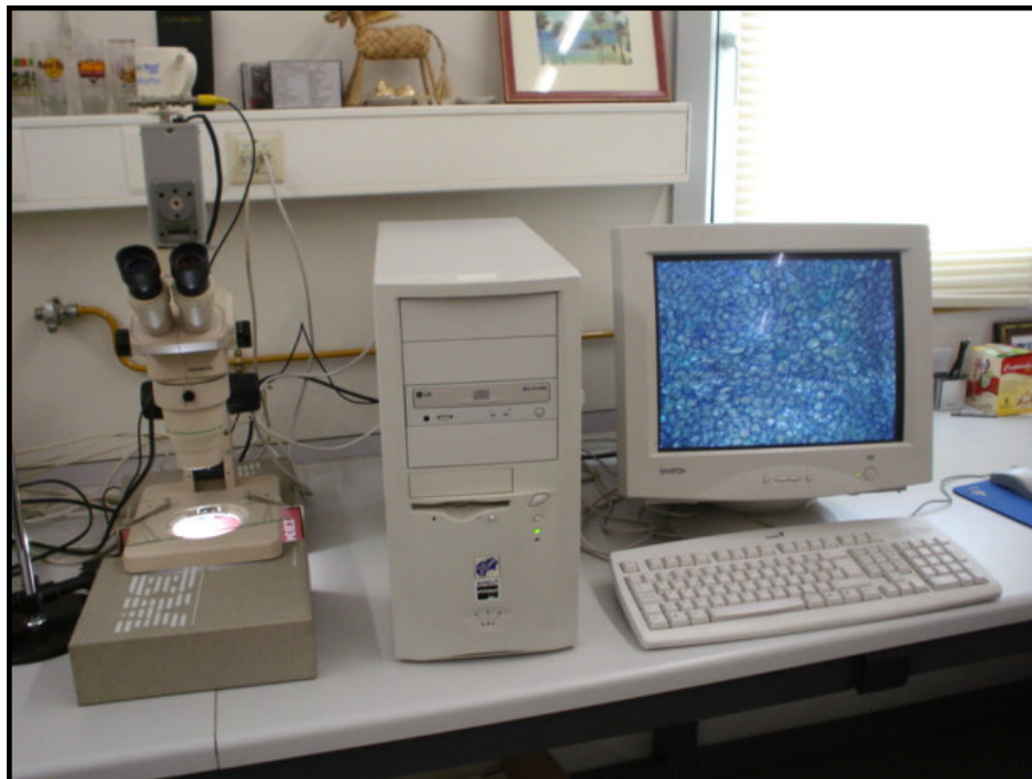
Figure 7.3. Equipment for microscopical observation with the stereomicroscope.
