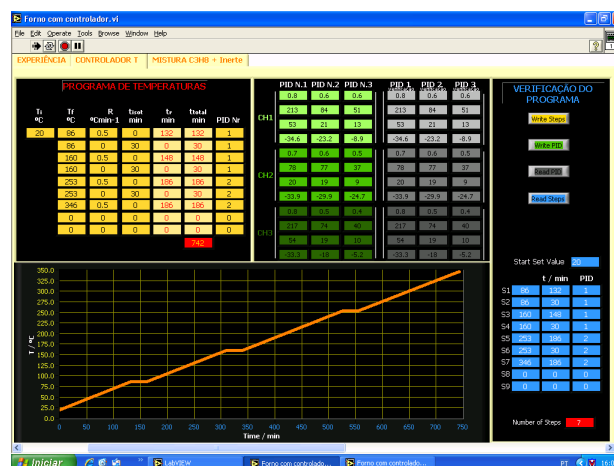
Figure B.6– Program developed for controlling the furnace - PID parameters input.
