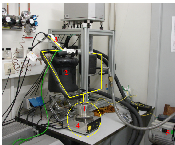
Figure B.10 – Picture of the magnetic suspension balance adapted for operation with water vapor.
