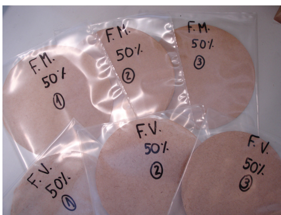
Figure C.1 – Example of supports made of cellulose+50 % inorganic fibers: pulp of virgin fibers (F.V.) and of treated fibers (F.M.); 1, 2 and 3 correspond to 60, 120 and 300 g cm -3 paper densities.
