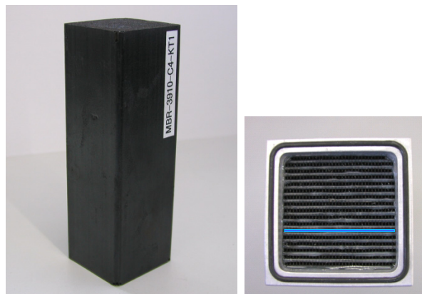
Figure B.14 – Monolith sent by Blue Membranes, Germany, on the left; top view of the monolith glued very each row. The blue line represents feed going in.
