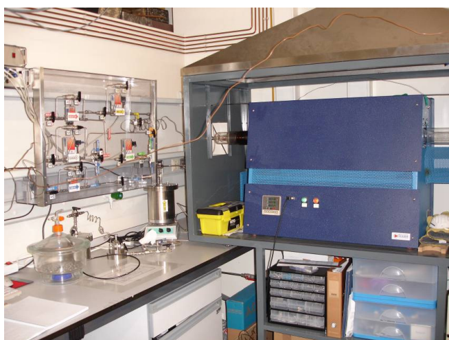
Figure B.4 – Global view of the CMSM pyrolysis set-up.
