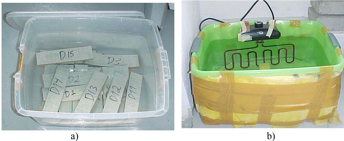
Figure 2 – a) Samples conditioned at room temperature; b) Samples conditioned at 50^{\circ}\text{C} ;
