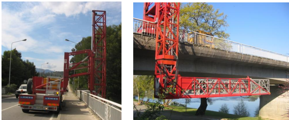
Figure 7.3 – View of the special vehicle used in the external inspection of the deck.
