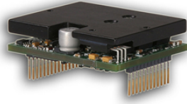
Figura 3.13: Driver Motores AMC DZRALTE – 012L80 [29]
