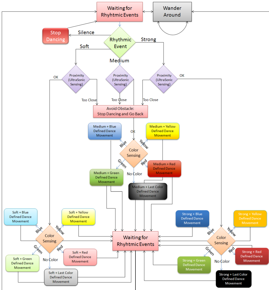
Figure 28 - Robot Control Module flow chart: processes and decisions involved in the robot control algorithm, inciting a different dance reaction to the occurrence of each rhythmic and sensorial event’s conjunction.
