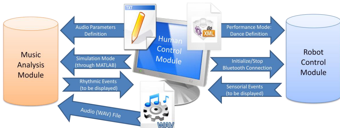
Figure 32 - Human Control Module (GUI) bi-directional interaction with the Music Analysis Module and the Robot Control Module .
