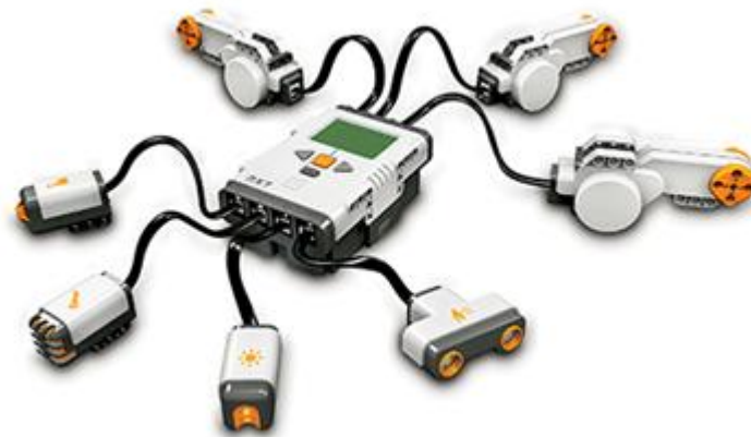
Figure 1 - Lego NXT brick and some of its sensors and servomotors.
