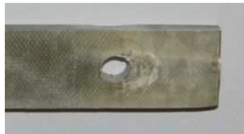
Figure 3.37: P-2-2 specimen after loading
