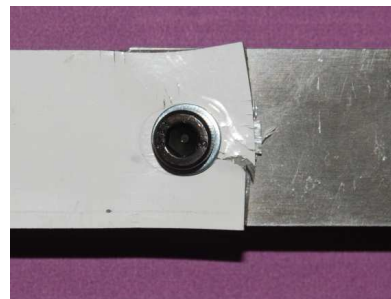
Figure 3.61: P-A-3-3 specimen after loading
