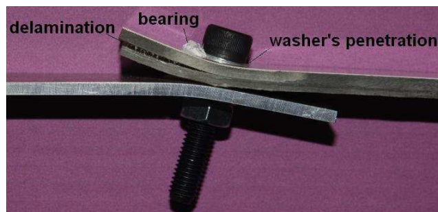
Figure 3.121: Aluminium-vinylester connection after being loaded
