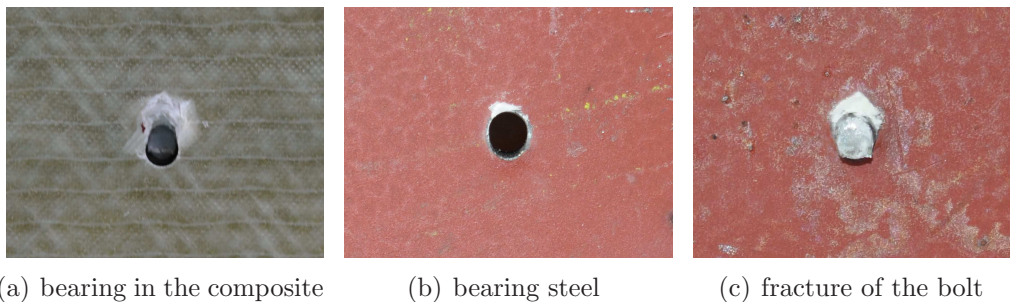
Figure 7.6: Failure modes of the multi-material sub-component
