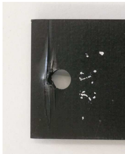
Figure 6.13: Shear specimen after loading
