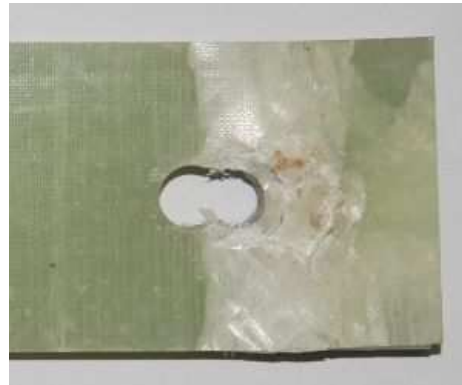
Figure 3.19: E-4-3 specimen after loading
