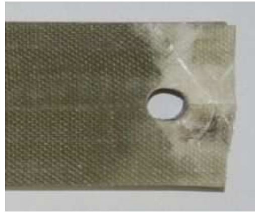
Figure 3.40: P-3-3 specimen after loading
