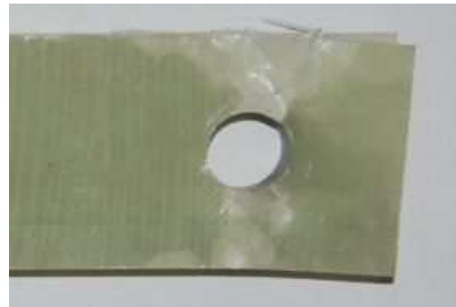
Figure 3.10: E-1-3 specimen after loading
