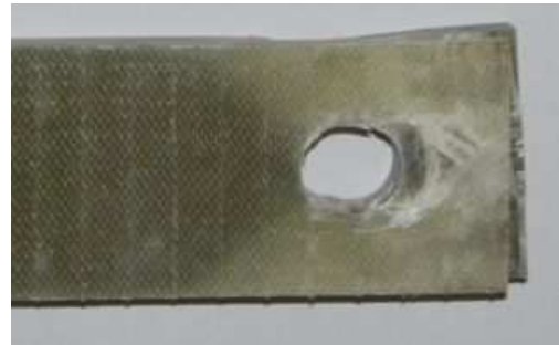
Figure 3.34: P-1-1 specimen after loading
