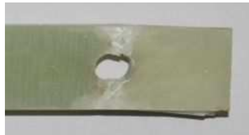
Figure 3.13: E-2-3 specimen after loading
