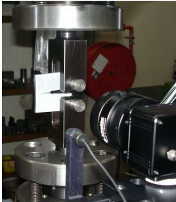
Figure 4.12: Equipment set-up during CT-CC tests
