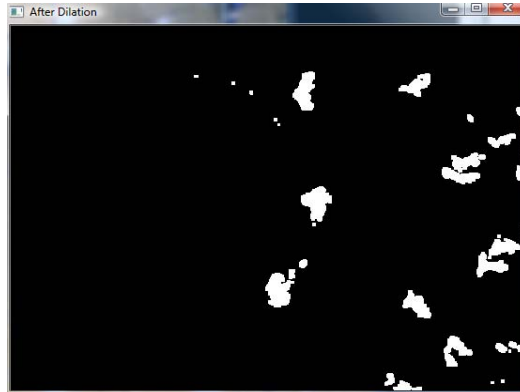
Figure 69 - Dilation process applied to the image
