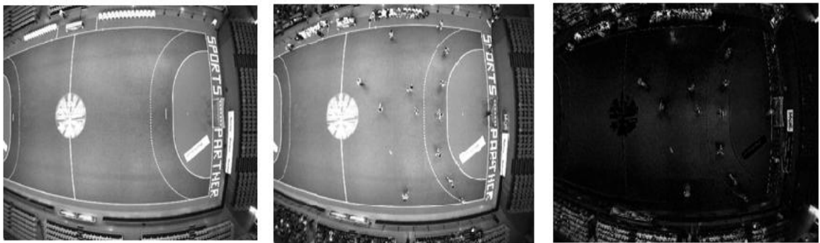
Figure 30 - Static Background Subtraction
