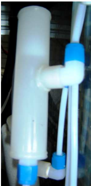
Figure 2.8 – Air trap placed before the membrane cell inlet.
