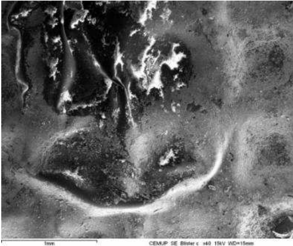
Figure 2.3 – View of the blistered carboxylic layer of membrane A (40 x).
