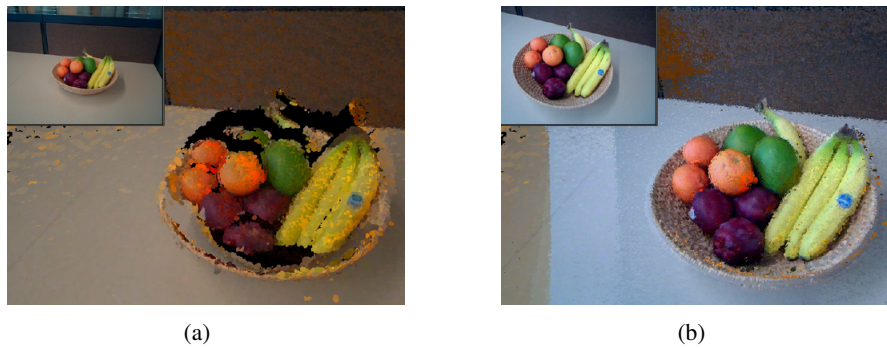
Figure 3.13: Surfel update demonstration in Henry et al. [10]. (a) Initial frame; b) Complete updated surfel with 95 RGB-D images.
