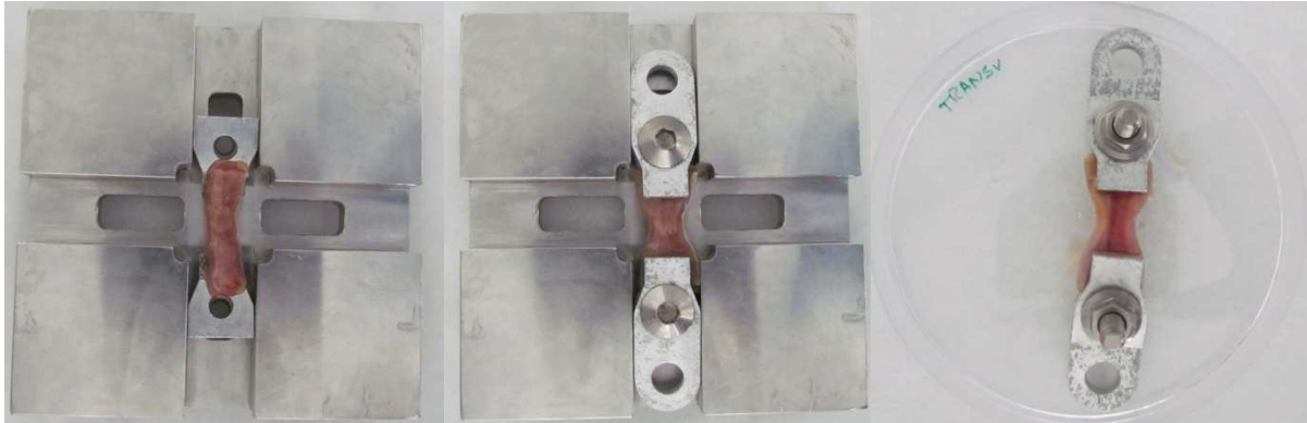
Figure 4.6 Assembly of a transverse abdominal uniaxial muscle specimen.
