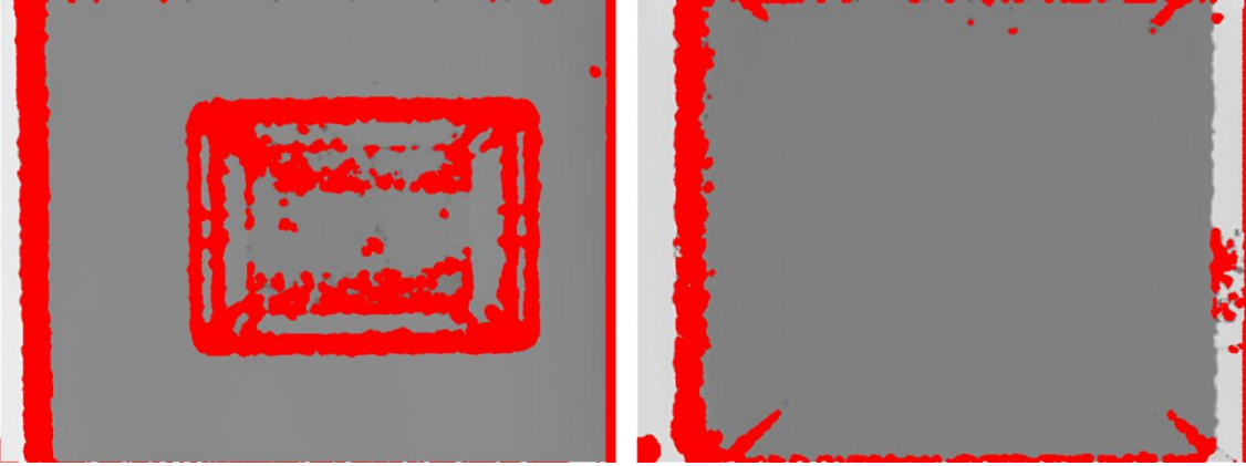
Figure 4.6 - Sample depthmap images of home-cage (left) and open-field (right) apparatus with unresolved areas marked red (pixels for which the Kinect does not return any depth value).
