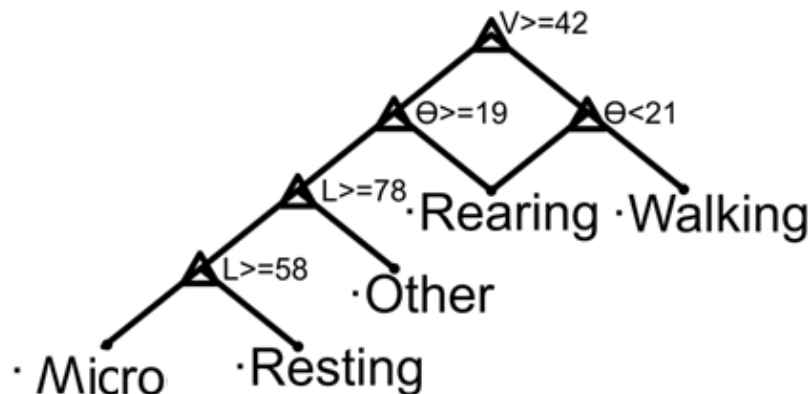
Figure 4.8 - Example classification based on a decision tree with three feature (mouse length (L, pixel), angle of elevation ( \theta , ^\circ ), principal velocity (V, \text{pixel}\cdot\text{s}^{-1} )).
