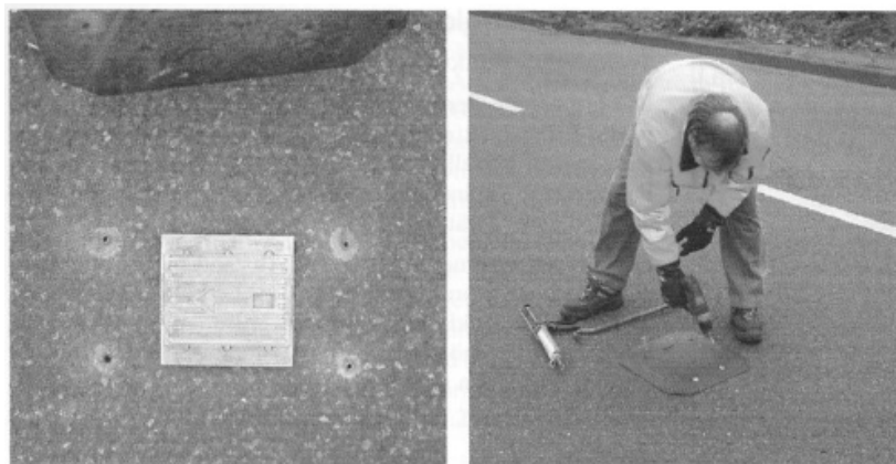
Figure 3.16 – Application of a magnetic sensor [3]
