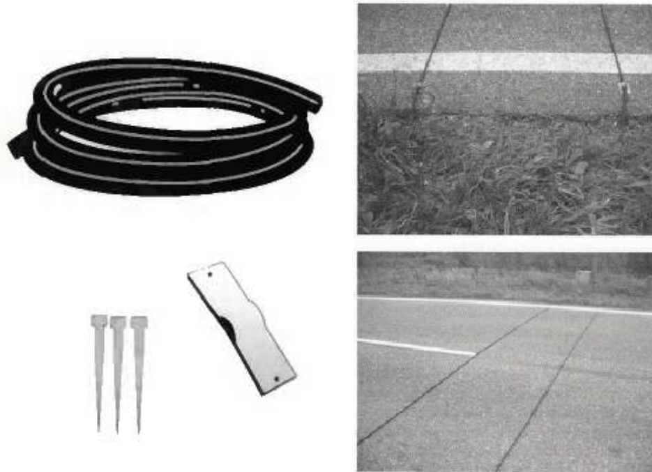
Figure 3.2 – Example of material used when fixing tubes, and its final presentation [3][7]
