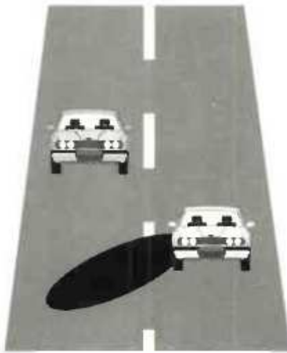
Figure 3.14 – Video system without marks in the pavement [7]
