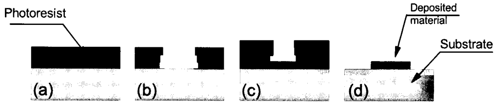
Figure 2.4: Schematic of lift-off process. The photoresist (a) is exposed to the laser light and the exposed areas removed (b). A material is then deposited (c) and, after lift-off of the photoresist by a chemical process, the layer is patterned (d).
